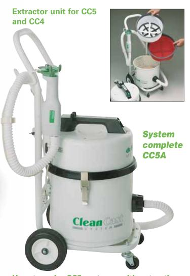
The four stage filtration system consisting of an easy to change disposable collection bag, two cloth filters and a micro filter. The micro filter retains 99.997% of all dust particles greater than 0.5 microns.
